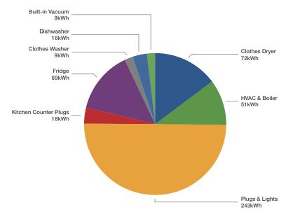
Figure 4. Percentages of energy consumed (in kWh) over the 59-day period for a total of 478 kWh.
