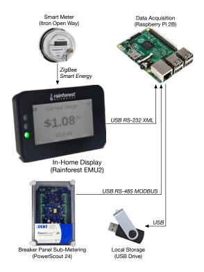
Figure 2. Diagram of the data capturing hardware/setup.
